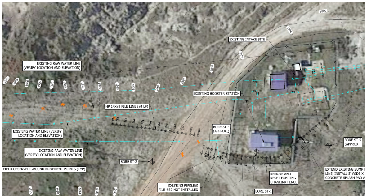
Figure 1. From Slide Area Pile Line Site Plan
